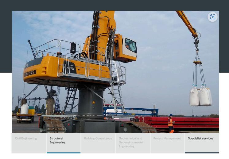
Structural assessment of suitability of existing quay to receive new cargo handling operating equipment and development of operational methods.
